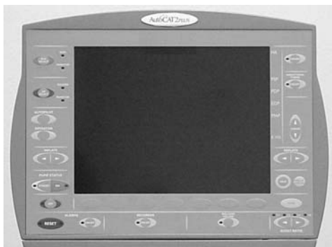
Figure 3.2: The AutoCAT®2 Series LCD and Control Function Keypad
