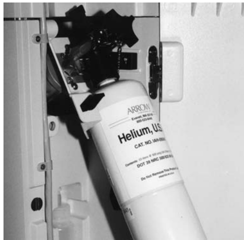
Figure 10.4: Helium Tank Installation with Disposable Tank
