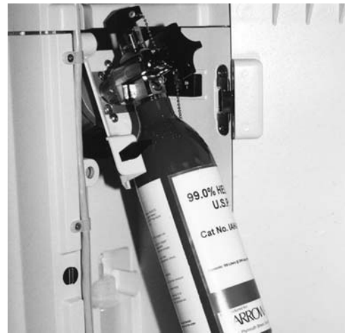
Figure 10.5: Helium Tank Installation with Refillable Tank >2000 psi
